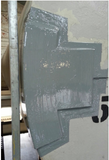
Belzona 1212 High-performance, rapid-curing, surface-tolerant epoxy repair composite suitable for wet and oily surfaces. Approved for contact with drinking water (e.g. WRAS).
