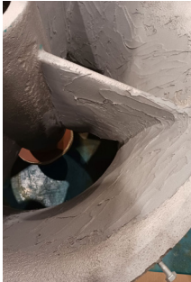
Belzona 1121 (Super XL-Metal) High-performance, extended working life, durable epoxy composite for the repair and rebuilding of metal components.
