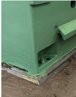
Belzona 7111 Pourable chocking/grouting material designed to spread evenly across uneven surfaces to endure physical and thermal shock.
