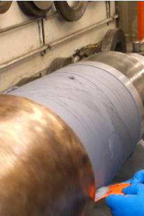
Belzona 1111 (Super Metal) High-performance, durable epoxy composite for the repair and rebuilding of metal components. Approved for contact with drinking water (e.g. WRAS, NSF/WQA).
