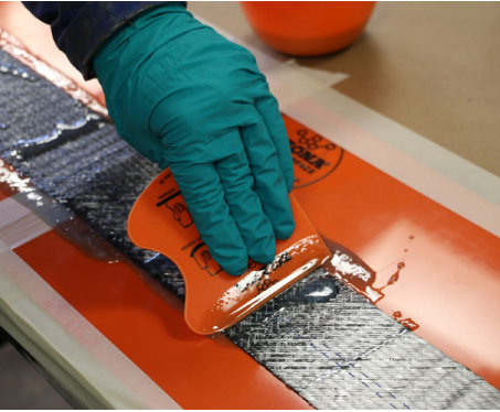
Belzona 1981 Low-temperature resin for application temperatures of 5°C (41°F) - 20°C (68°F) and operating temperatures up to 60°C (140°F).
