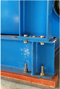
Belzona 7111 Pourable chocking/grouting material designed to spread evenly across uneven surfaces to endure physical and thermal shock.
